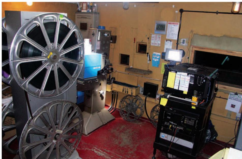
retired, the most used piece of equipment is a NEC NC 800C digital projector working with a Doremi DCP 2000 digital cinema server. Sound is being delivered by a Dolby CP65 processor with SST amps.
