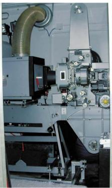
The second unit has either another Victoria 8 or a highly adapted Kalee 21 with an ISC curved gate and analog reader. The second unit uses either a 35 ft wide X 15ft scope screen or a 25ft X 19'10" Academy Screen which is electrically raised and attached to the side of a lorry, this has a 3 kilowatt Kinoton lamphouse, both units have digital sound using the Dolby CP500 system.
